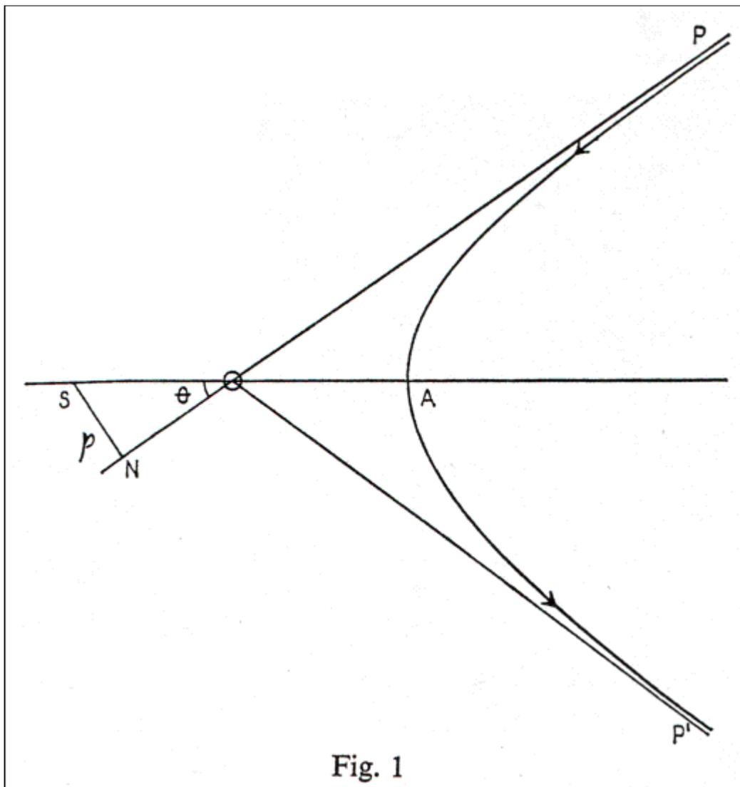
on escaping the atom is  $OP'$ .  $OP$  and  $OP'$  make equal angles with the line  $SA$ , where  $A$  is the apse of the hyperbola.  $p = SN =$  perpendicular distance from centre on direction of initial motion of particle.
